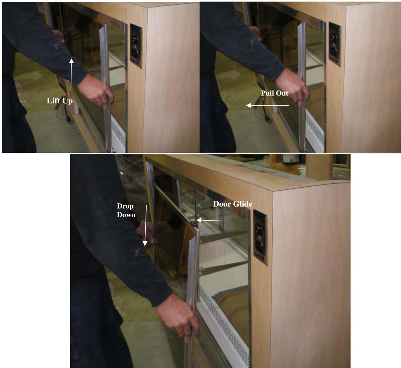
Once doors have been removed from display case. You will note that there are a total of four nylon glides. Two glides are installed on the top of the door and two glides are installed on the bottom of the door.
